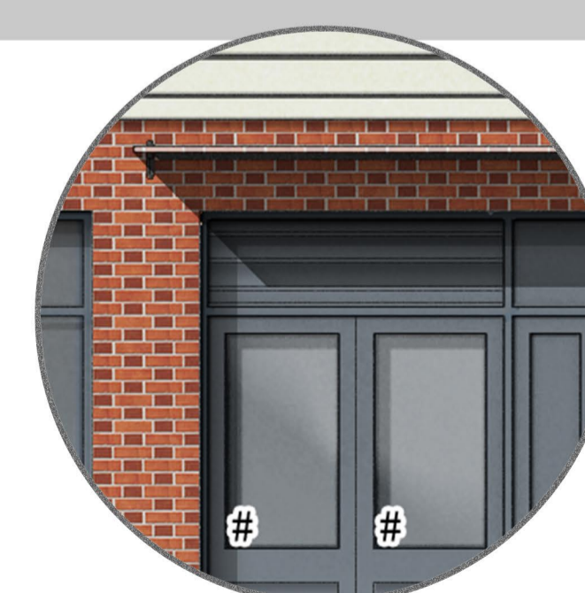
Tiered stone horizontal banding around the building to visually differentiate to ground level commercial frontage from the residential properties above
