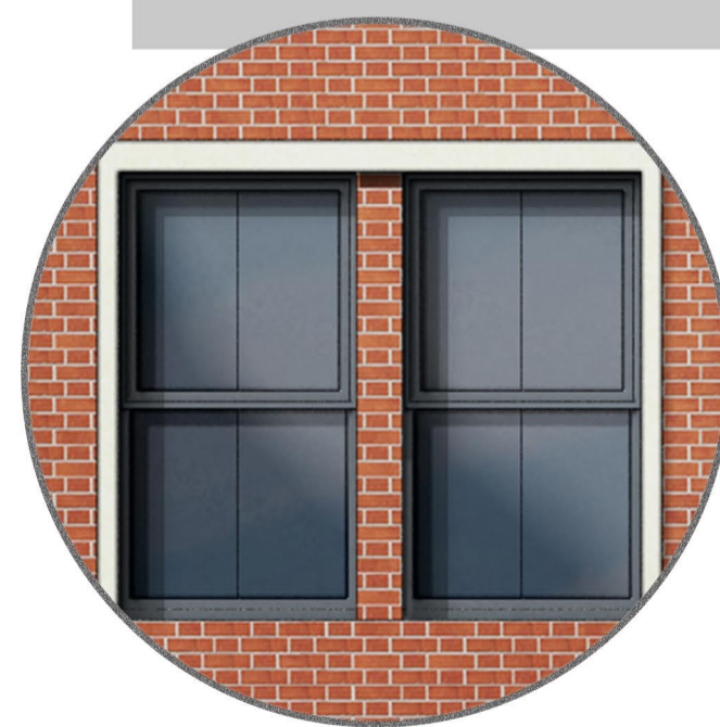
Stone surrounds around all first and second storey windows with a contemporary low profile grey coloured window
