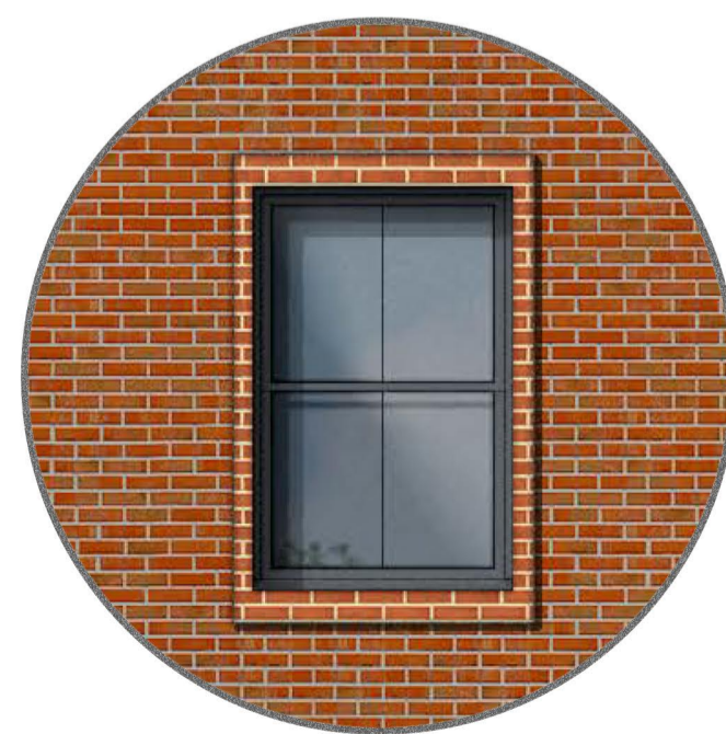
Feature brick surrounds on front elevation windows, to compliment the main brick with a contemporary low profile grey coloured window
