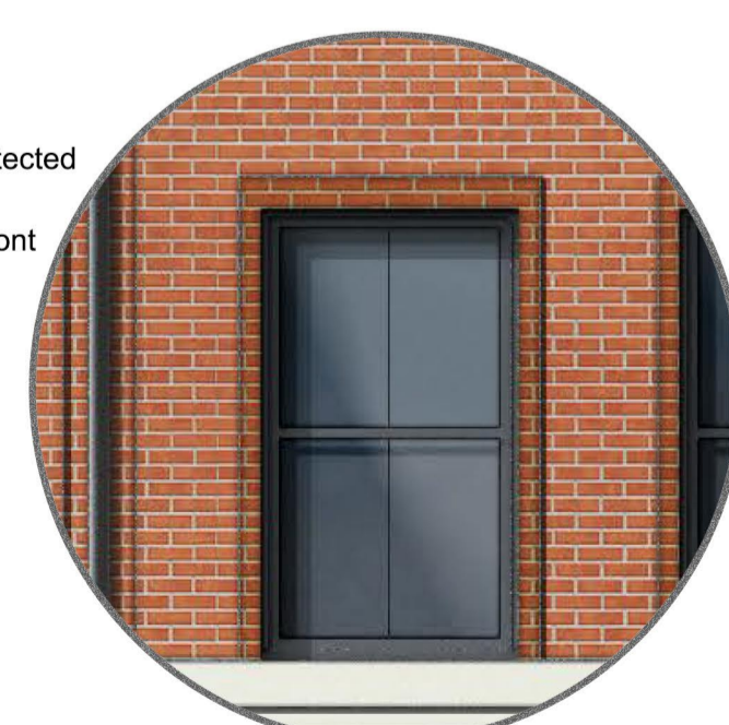
Brick surrounds around all first and second storey windows inset with a contemporary lowprofile grey coloured window
