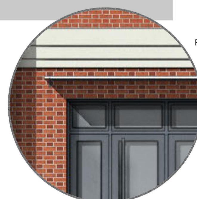
Tiered stone horizontal banding to visually differentiate ground level commercial frontage from the residential properties above
