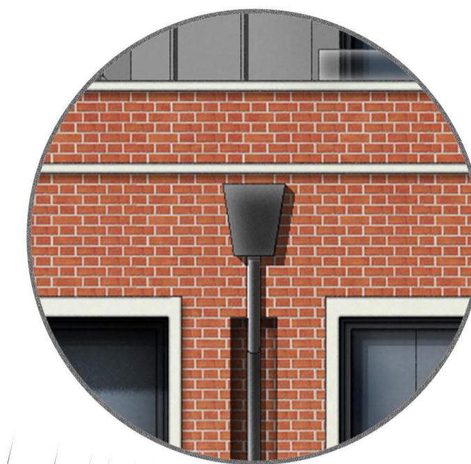
Rain water pipes recessed back into brick through a stepped channel
