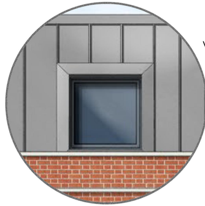
Contemporary mansard zinc seamed roof
