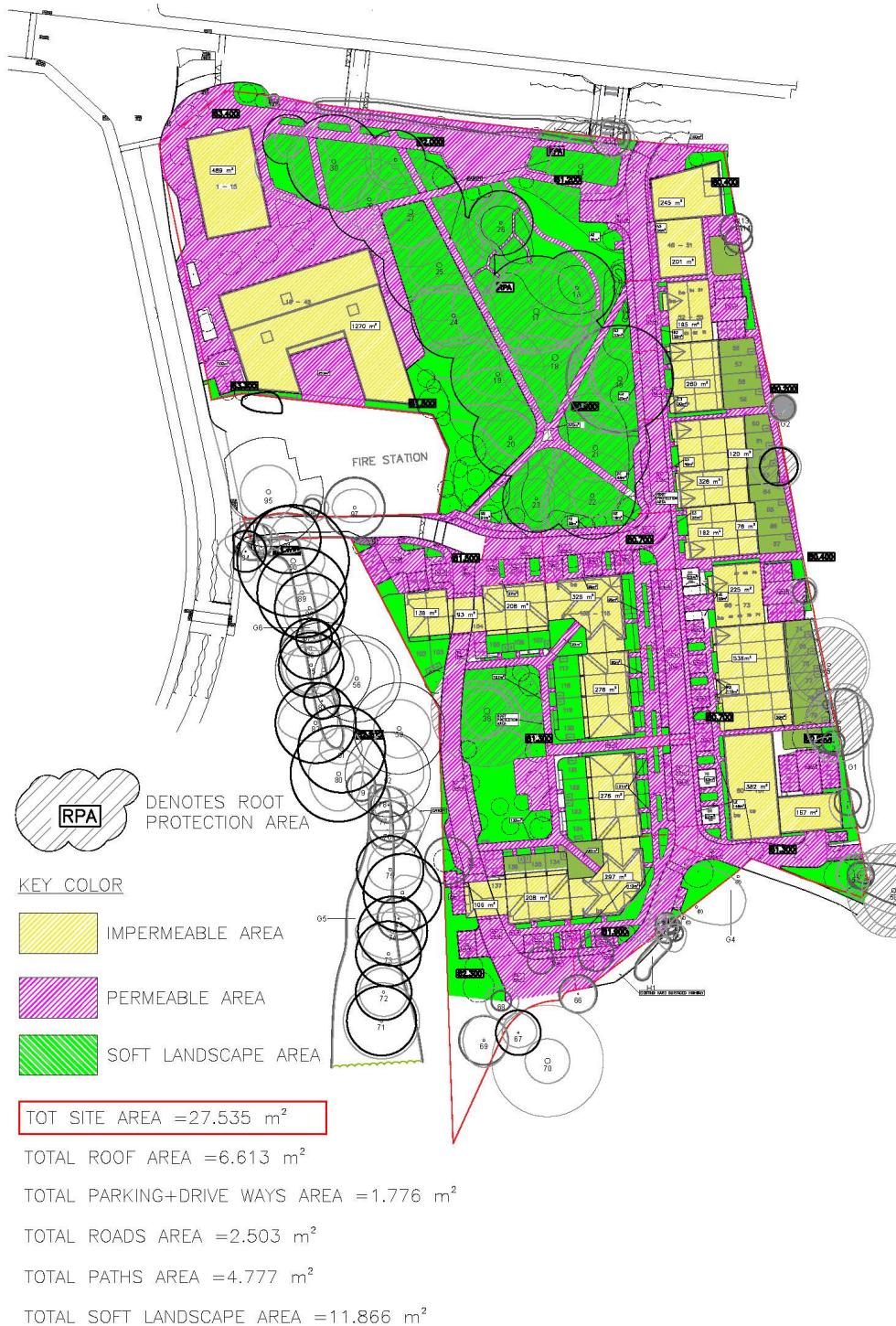
Figure 7 Development layout surface Areas submitted in Appendix D of 21146-REP01-FRA dated May 2022
